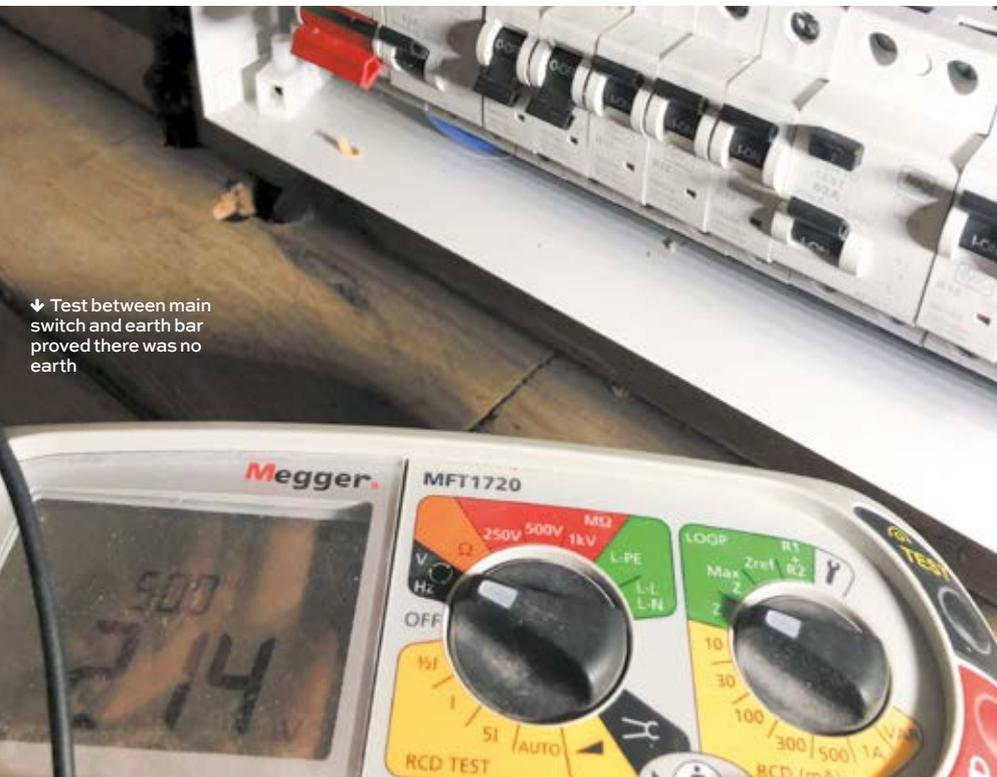
↓ Test between main switch and earth bar proved there was no earth
